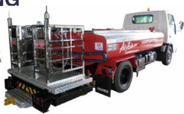
Water tank and all fittings are made from food grade stainless steel material and designed for supply of clean water to the aircraft
